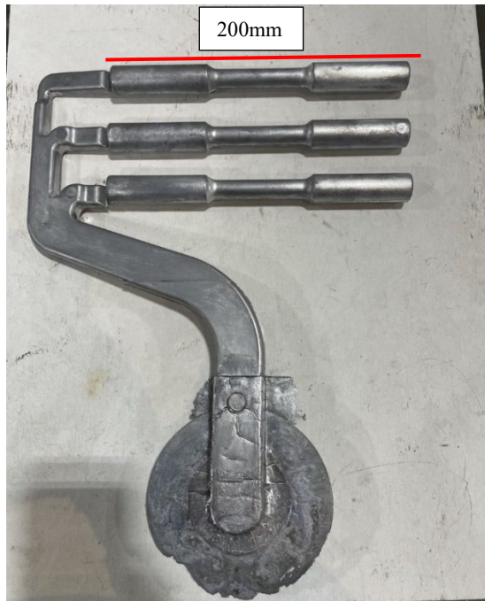
Figure 2. Tensile bar die casting in which hot shear specimens were taken from the middle of the reduced section of the tensile bars.
